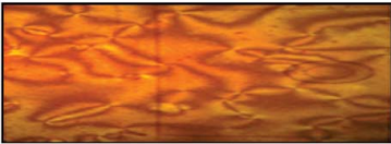
(g) Schlieren texture of nematic phase Binary system VII (69.82 mole%)
